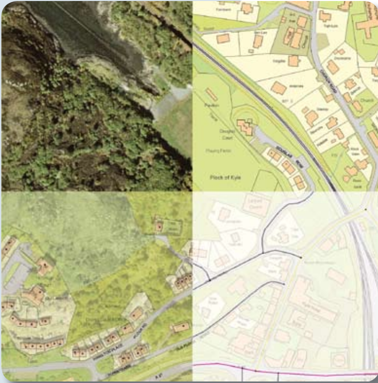
OS MasterMap is a digital representation of the real world containing more than 450 million uniquely identified geographic features. It is updated daily as a consistent framework for the referencing of geographic information in Great Britain. OS MasterMap is available in four data layers: Topography Layer, Imagery Layer, Integrated Transport Network Layer and Address Layer. Courtesy of Ordnance Survey.
